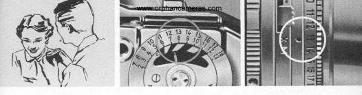
**SET THE EXPOSURE VALUE** on the camera by depressing the tab on the lens opening ring and moving the red e-v index dot to the indicated value. The dot can be set either on the values or halfway between them. Turn the shutter speed ring to a different setting if the lens opening ring will not turn far enough for the correct exposure value.
