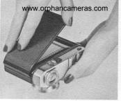
4 The exposure counter shows how many pictures are remaining on the film. It must be set before the back cover is replaced. For 20 exposure roll of film, move setting dial (just above film track) with your fingertip until counter shows red 22. With a 36 exposure film, turn until counter shows red 2.
